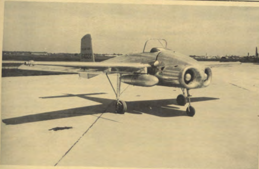
LEFT— BELL'S EXPERIMENTAL VERTICAL RISING AIRPLANE, X-14, takes off and lands in conventional horizontal position. It is jet-powered.
